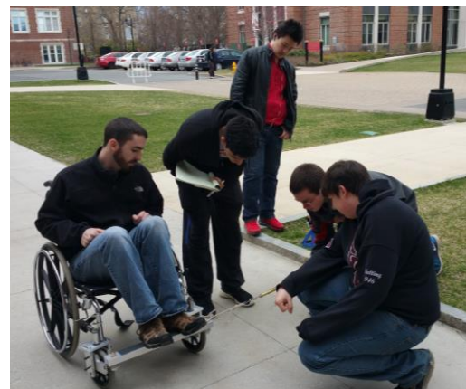
Figure 4. Measuring the horizontal force required to operate the turning bar on design 1.
