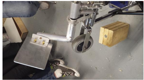
Figure 2. Design 2 used a single rotatable footrest and a toothed rubber belt to rotate the front caster.
