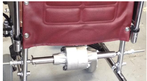
Figure 3. Removing the differential connecting the two rear wheels allowed the wheelchair to fold.
