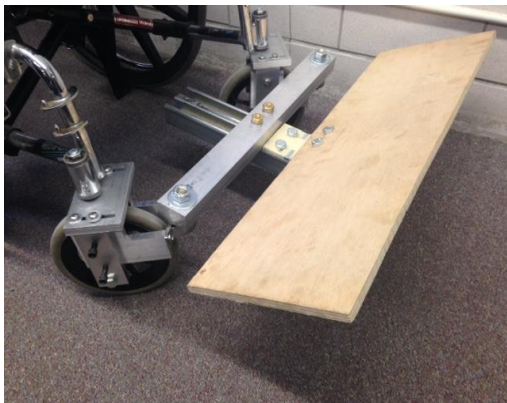
Figure 1. Design1 utilized a steering bar with an optional wooden footrest.
